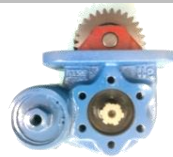
PTO shaft is rotating to the right will turn the pump on the left.
